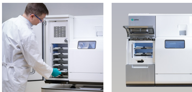
Fig 18. Sample hotel in Biacore 8S+ can hold up to twelve 96- or 384-well microplates and Biacore 8S holds up to four microplates.
