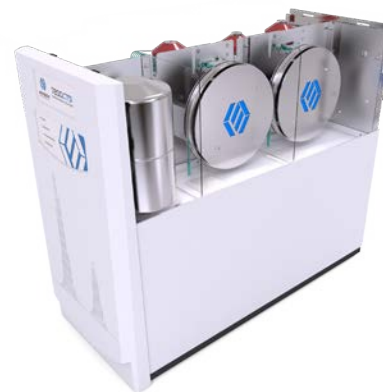
Figure 6 - The two Multi-Capillary Column Trapping Stages are shown above: Stage 1: Trap; Stage 2: Focus. Simple fans are used to cool traps down to 35°C. No complicated electronic cooling makes it easier to operate and maintain by the laboratory chemist.
