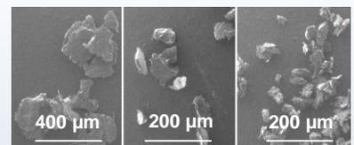
Grinding temperature at 25 °C
