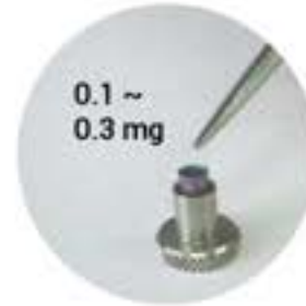
Sampling Placed in a sample cup
