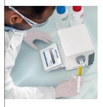
Measure density, refractive index as well as many related values, such as specific gravity, % alcohol, or Brix of your samples quickly and reliably. No need for table lookup or conversions: the instrument performs all necessary calculations.
