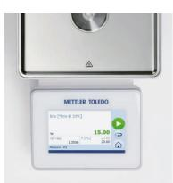
Simplify your routine measurements and instantly identify acceptable samples by setting up a range of tolerable limits for your sample. Color-coded results allow the user to quickly identify if a measurement is within or out of limits.
