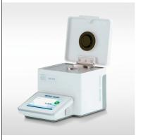
For users who require accuracy and ease of use, digital refractometers are the perfect choice, combining simple and quick measurements with an intuitive workflow. A high-resolution optical sensor rapidly measures the refractive index of your sample.
