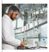
Measure density near production line: The new measuring cell design minimizes the influence of external mechanical vibrations and allows for precise results even in turbulent environments.
