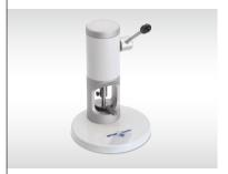
The press allows the pan to be sealed very easily. Under the pressure of the plunger the pan is cold welded, hermetically sealing with the lid. After changing plunger and die you can use the press for other crucibles.
