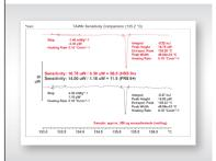
A quantum jump in sensor technology enables us to offer the highest sensitivity sensors available in DSC instrumentation and allows you to detect the weakest thermal effects. The signal-to-noise ratio, an important instrument parameter, is determined by the number of thermocouples and their specific arrangement.
