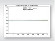
Our revolutionary star-shaped arrangement of thermocouples around the sample and reference crucibles completely compensates any possible temperature gradients. This guarantees flat baselines and reproducible measurement results.
