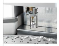
The sample robot can remove the protective crucible lid from the crucible or can pierce the lid of hermetically sealed aluminum crucibles immediately before measurement. This unique feature prevents the sample from taking up or losing moisture between weighing-in and measurement. It also protects oxygen-sensitive samples from oxidation.
