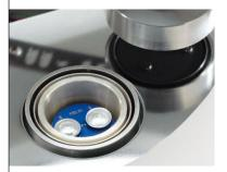
The automatic furnace lid opens and closes the furnace chamber at a keystroke or when actuated by the SmartSens infrared sensors. Manual removal and replacement of the furnace lid is no longer necessary. The measurement cell is effectively isolated from the environment thanks to its optimized design with three superimposed silver lids and its heat shield.
