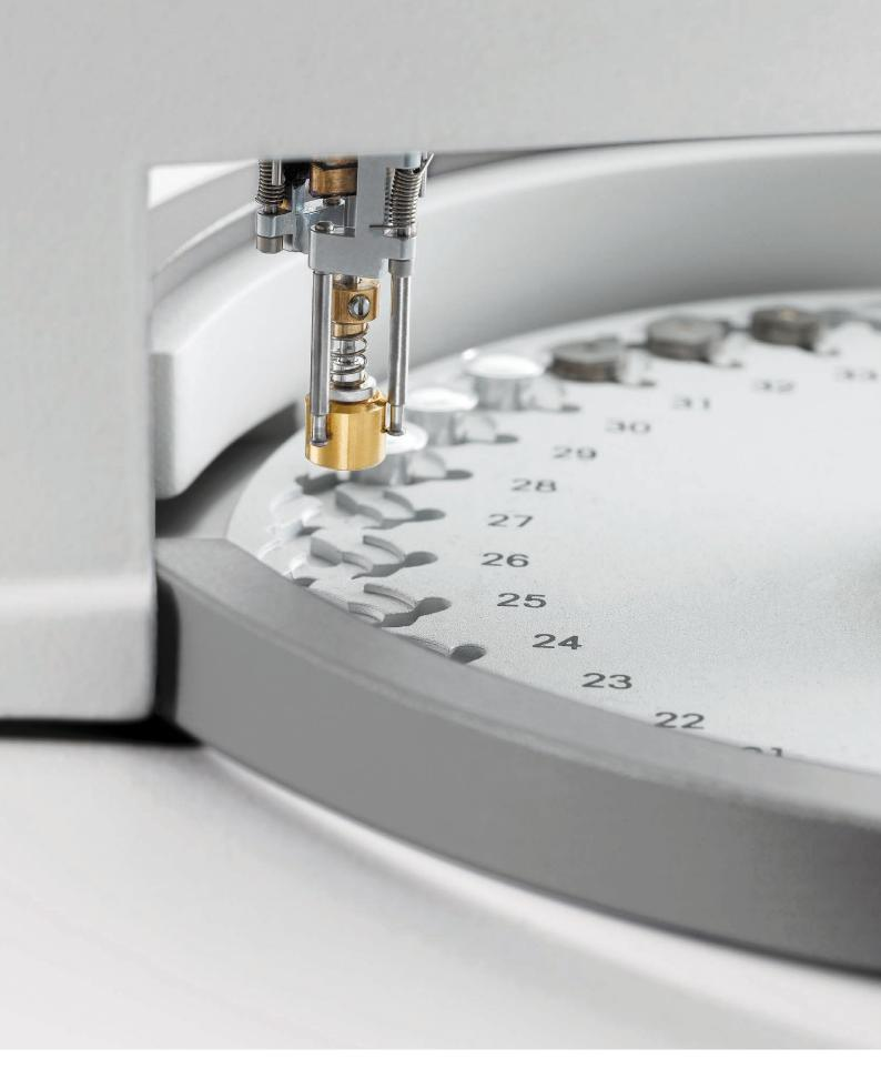
All our DSC models can be automated. The sample robot can process up to 34 samples even if every sample requires a different method or a distinct crucible.
