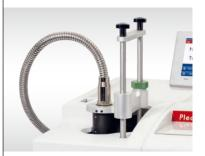
The photocalorimetry accessory for the DSC allows you to characterize UV curing systems. You can study photoinduced curing reactions and measure the effects of exposure time, UV light intensity and temperature on material properties.
