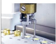
The universal gripper can handle all types of METTLER TOLEDO crucibles.
