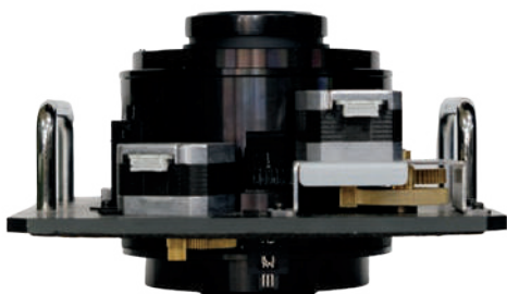
Fig 6. The large aperture Fujifilm lens of the Amersham ImageQuant 800 imager.
