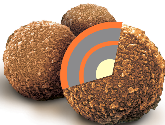
Fig 1. SEM image showing the cauliflower-like surface of the Sera-Mag Magnetic SpeedBeads. The surface dramatically increases the overall surface area available for binding.
